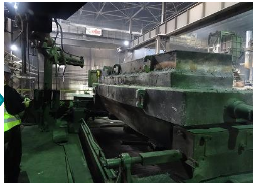
3. Tundish (Molten metal is poured into the mold to purify "Billet".)
