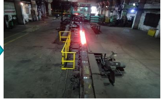
4. Heating furnace (To heat 'Billet' by using Coal gas (1150°C- 1250°C) )
