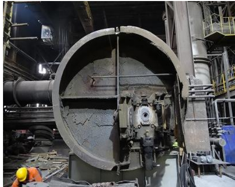
2. Ladle (To heat up to 1200°C and stir)
