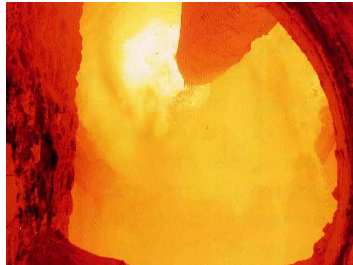
Inside view of Rotary kiln operating at a very high temperature of 1450 °C
