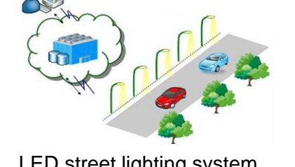
LED street lighting system with wireless network control, MinebeaMitsumi, Cambodia
