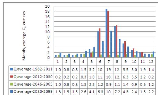
**Figure 3.35.** Current (1982-2011) and projected in future monthly average discharge values of the Kharkhiraa River at Tarialan hydro-station, ECHAM5-GCM, A1B (2012-2030, 2046-2065, 2080-2099)
