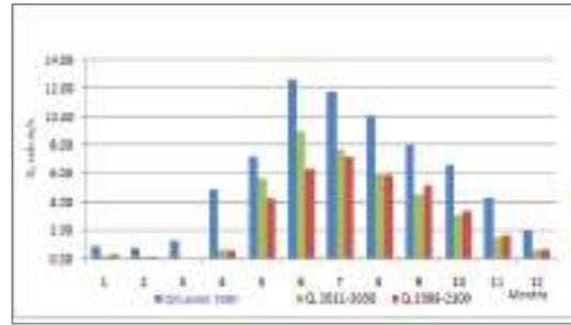
**Figure 3.26** Current (1980-2000) and projected in future monthly average discharge values of the Buyant River, ECHAM5-GCM, A1B (2011-2030, 2080-2099)
