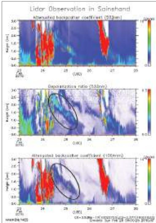
**Figure 3.59** The transported dust layer in the air over Sainshandon February 24-25, 2010.
